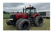
2010 Case IH 335 Magnum Tractor, MFWD, 3PT With Quick Hitch, 5 Remotes, PTO, 520-85-R46 Rear Duals, 480-70R34 Front Duals, 18 Front Weight, 8.9L 6-Cylinder Diesel Engine, 330 Hp, has 100-HP Chip added, 19-Speed Powershift Trans, Deluxe Cab, has Trinble Autosteer, it is also wired for Case IH Autosteer, primarly used for planting and grain cart, 5628 Hours Showing, S/N: ZARZ07575 ~ SERVICED AND FIELD READY
