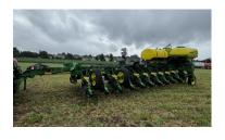
2013 John Deere 1770 NT Planter, 24-Row, CCS Seed Delivery, Precision 20/20 Monitor, Corn & Bean Plates, Row Shut Off, 450-Gallon Liquid Fertilizer, Martin Till Row Cleaners, In Furrow Fertilizer Tubes & 2x2 Fertilizer Discs, Stored Indoors, includes skid of extra parts, S/N: 1A01770CHEM755718
