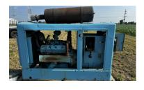
International Harvester Engine with Onan Generator, Engine Model: G549, Engine S/N: 132121, 8-cylinder gas powered, Onan Generator Model: 85.0 KR-15R, Single or 3 phase, Single -> 57 KW 3PH -> 85 KW, 247 Hours Showing
