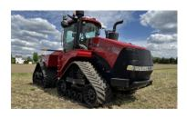
2022 Case IH 500 Quadtrac Tractor, 6 Remotes, PTO, 30" Tracks, 500-Hp, 12.9L 6-Cylinder Engine, 16F Powershift Trans, Autosteer, Deluxe Cab, AFS Connect, 664 Hours Showing, S/N: JEEZC500ENF504377 ~ SERVICED AND FIELD READY
