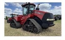
2012 Case IH 550 Quadtrac Tractor, 6 Remotes, PTO, 30" Tracks, 12.9L 6 cylinder diesel engine, 550 Hp, 16 Powershift Trans, Autosteer, Deluxe Cab, Tracks replaced 2 seasons ago, new bogies, seals, bearings 1 season ago, 4982 Hours Showing, S/N: ZCF129458—SERVICED AND FIELD READY
