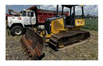
John Deere 650J LGP Crawler Dozer, PIN: T0650JX132507, 28" Wide Tracks, 10' Blade, Rockland Root Rake Model: BR, Hydrostatic Transmission, 6-way blade, 90 hp, all new undercarriage approx. 2 years ago (approx 200 hours ago): chains, sprockets, bogie wheels, idlers, track pads. 4553 hours showing, S/N: 6815401
