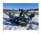
DMI 3200 ANHYDROUS APPLICATOR, S/N: 701005, 11-KNIFE, NO TANK, 3-POINT
