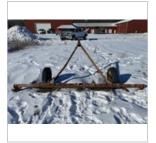
PORTABLE TOOL BAR, 93", EXTENDABLE, PIN HITCH
