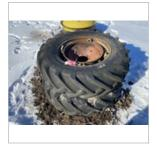
GOODYEAR 14.9-28 TIRES & RIMS WEATHER CRACKED, 8-BOLT RIMS
