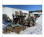
TOWABLE TANDEM AXLE SPRAYER, 1000-GALLON ALUMINUM TANK, 60' BOOM FOAM MARKERS, 13.5-16.1 TIRES
