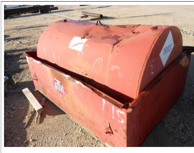
Empty skid tank AST on the subject property.
